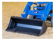
High Capacity Loader 2 Large Diameter Lift And 2 Large Diameter Curl Cylinders Enable 1,007 lbs. Lift Capacity
