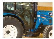
Standard Right-Side Cab **Door With Steps Provides Additional Access** To The Operators Platform
