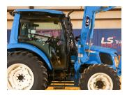
*Right-Side Door And Steps* Provides Access To Both Sides Of The Cab
