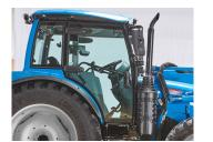
Right-Side Cab Access Enables Operators To Access Both Sides Of The Cab (Door And Steps)
